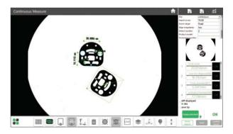
■ Measuring result can be stored automatically. OK items and NG items can be counted automatically.
