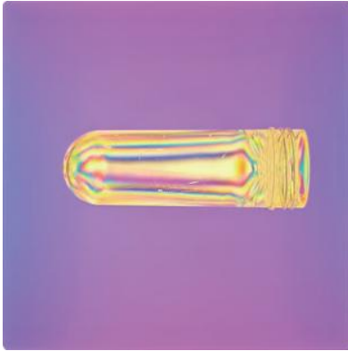
stress patterns of PET bottles measured by PSM-S02-U at 0° and 45° white light
