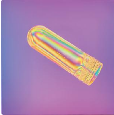
stress patterns of PET bottles measured by PSM-S02-U at 0° and 45° white light
