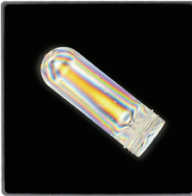
stress patterns of PET bottles measured by PSM-S02-U at 0° and 45° white light
