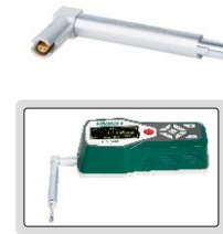
deep groove probe (optional), part no. ISR-C002-DGP
