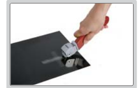
step 1: make grid cutting on surface
