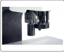
spectral confocal sensor (optional) measuring accuracy is .0002"
