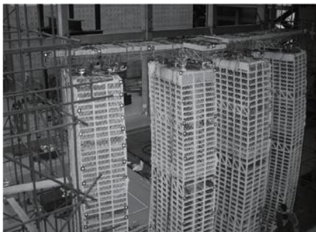
deformation monitoring of large building vibration test
