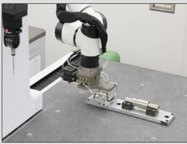
The robot automatically places the workpiece on the CMM station for automatic measurement
