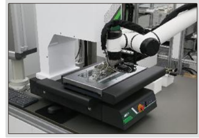
The robot automatically places the workpiece on the CNC vision measuring station for automatic measurement
