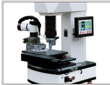
The robot automatically places the workpiece on the hardness tester station for automatic measurement
